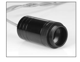
11. Insert the entire assembly, C-mount adapter first, into one of the 30mm cage plates from step 5. Lock into place using M3 set screws.
