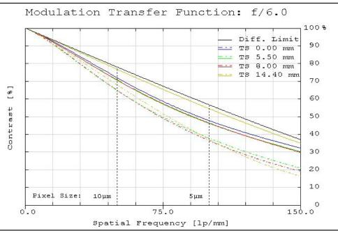
Figure 3: Image space polychromatic diffraction FFT Modulation Transfer Function (MTF) for  $\lambda$  = 486nm to 656nm. Included are Tangential and Sagittal values for field points on center, at 70% of full field and at the maximum sensor format. Solid black line indicates diffraction limit determined by f/#-defined aperture. Frequencies corresponding to the Nyquist resolution limit of pixel sizes are indicated.
