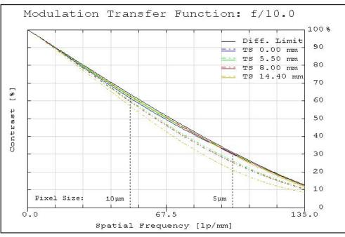
Figure 5: Image space polychromatic diffraction FFT Modulation Transfer Function (MTF) for  $\lambda$  = 486nm to 656nm. Included are Tangential and Sagittal values for field points on center, at 70% of full field and at the maximum sensor format. Solid black line indicates diffraction limit determined by f/#-defined aperture. Frequencies corresponding to the Nyquist resolution limit of pixel sizes are indicated.
