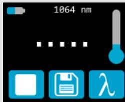
**NOTE:** At any time during the measurement sequence, you can press the STOP
