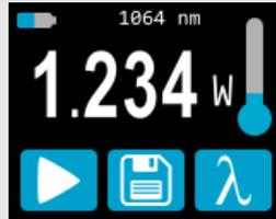
6. The reading will stay on the display until the next measurement, even if you turn the device off and on again.
