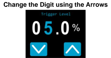
The adjusted level is saved automatically when exiting this screen
