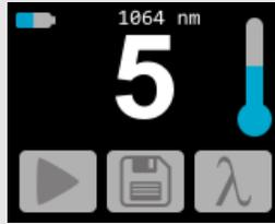
5. Once the countdown is finished, the measurement will appear. You can remove the device from the beam path.
