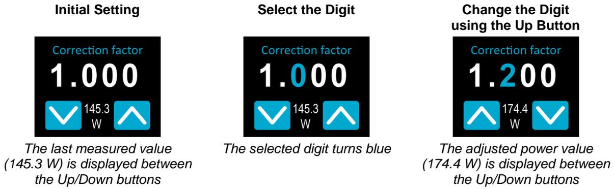
Once the value is entered, press the On/Off/Settings button to exit the menu and automatically save your new settings.
