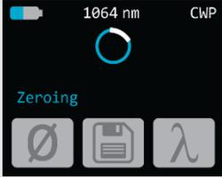
4. When the process is complete, the device returns to the measurement screen and you are now ready to make an accurate measurement.
