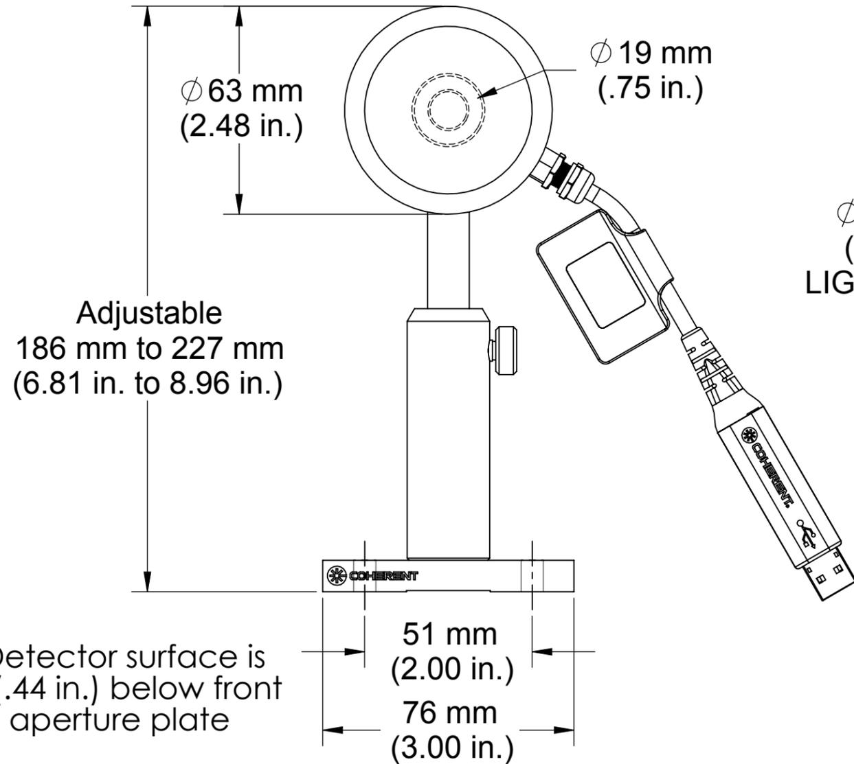
Note: Detector surface is 11 mm (.44 in.) below front face of aperture plate
