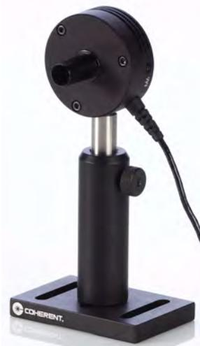
The Quantum EnergyMax series consists of three different models that provide very low pulse energy measurement down to 20 pJ. Two of the models (J-10SI-LE and J-10SI-HE) incorporate a Silicon photodiode, and one model (J-10GE-LE) incorporates a Germanium photodiode. All three models contain large 10 mm clear apertures and operate at repetition rates from single pulse up to 10 kHz.
