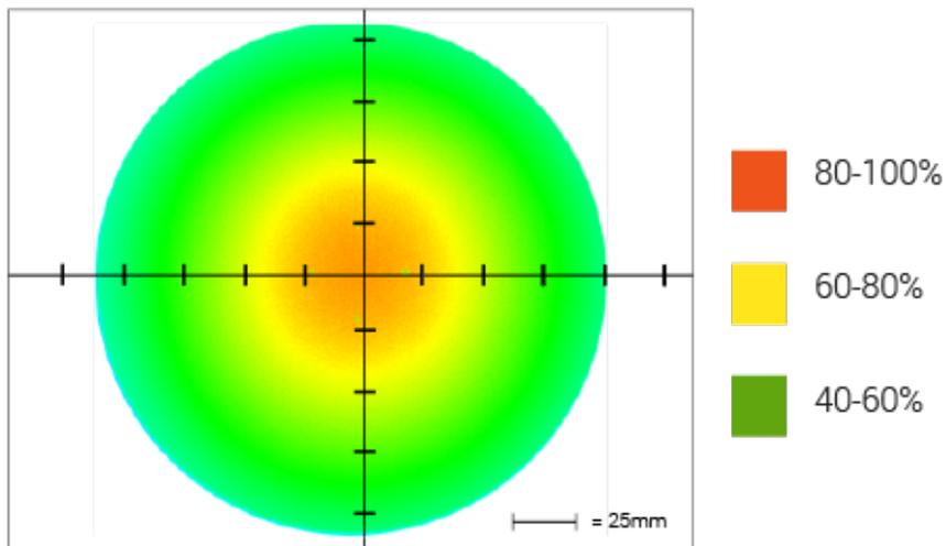
Optical measurement taken using RL208M-100WHIIC @ 300mm
