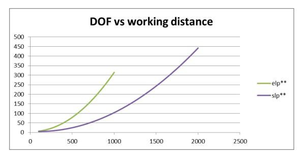
The graphs above show the values for line width and depth of focus of a 670 nm laser. To get the values for a different wavelength the factor from the table has to be multiplied by the values from the graphs.
