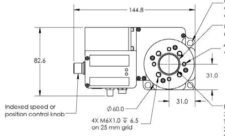
Mounting holes for \_M6 or [1/4"-20] screws at 50 mm [2"] grid spaced around centre of rotation
