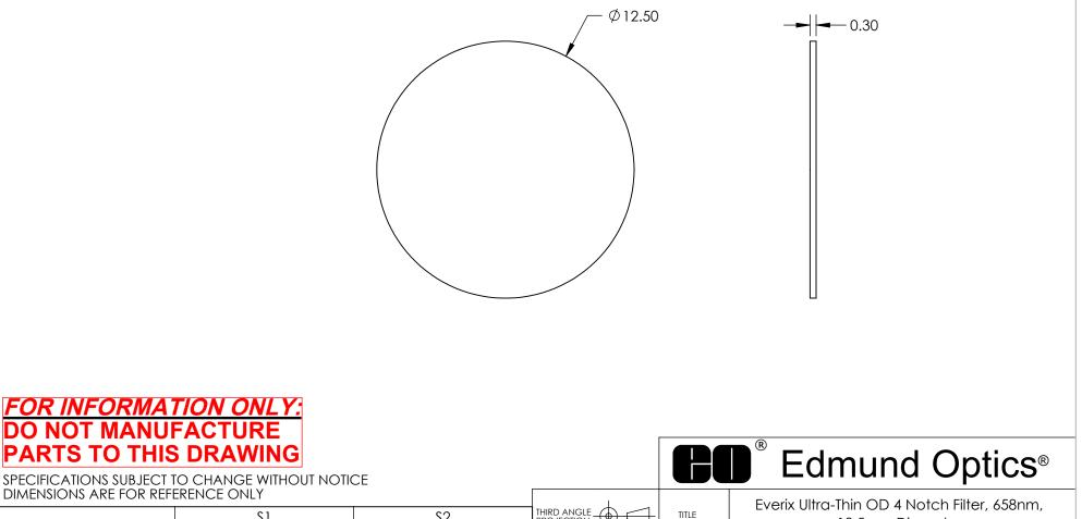
DIMENSIONS ARE FOR REFERENCE ONLY THIRD ANGLE S2 S1 12.5mm Diameter PLANO PLANO ALL DIMS IN DWG NO mm Ø11.25 Ø11.25 23681 CLEAR APERTURE
