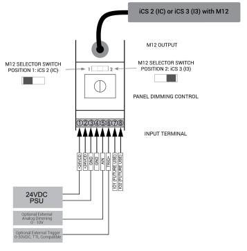
Note: When using external sources for triggering or analog dimming, it is important to use common ground returns for all supplies. A second ground pin is located on Pin 4 of the DCS-MP for this purpose.
