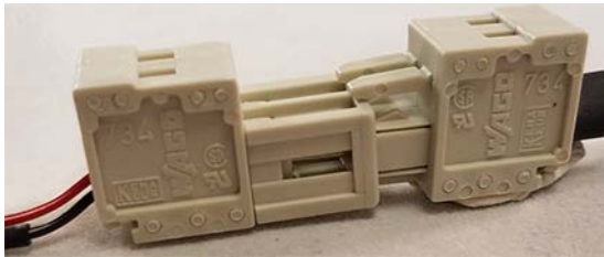
Figure 2-17. Connect Terminal Plug Ends
