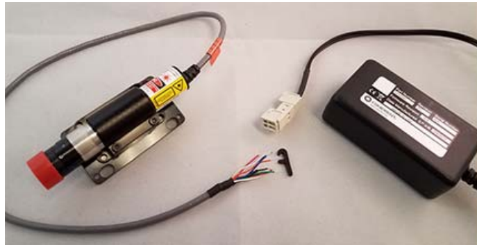
Figure 2-11. Flying Leads Example — Connector to Power Supply
