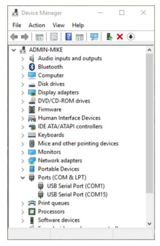
■ In this example there are two serial ports available (COM1 and COM15), which are both USB adaptors.
